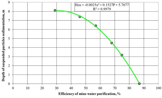
Figure 4. Dependence of the depth of suspended particles sedimentation on the value of the mine water purification efficiency
