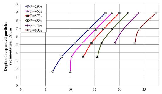
Figure 3. Dependences of the suspended particles sedimentation depth on the distance at which they can precipitate
