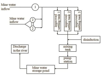
Figure 1. Improved technological scheme of mine water drainage for the "Stepova" coal mine: 1 – auxiliary shaft; 2 – drainage wells
